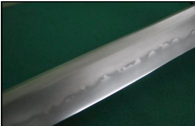
Japanese Katana - 1050 Steel, charcoal heat treated, clay hardened, FeCl etch Al Shannon, Wildfire Forge, Cranbrook, BC
